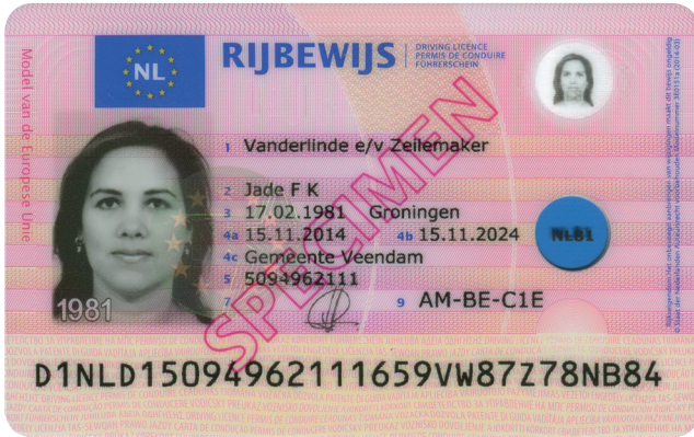
Figure 2: (Top left) European driving licence with laser engraved data, hologram patch, MLI, 1-line MRZ and a personalised window element (green patch on the right hand side of the card).
