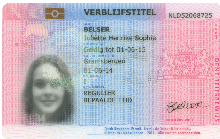
Figure 1: European residence permit with laser engraved 3D image, additionally protected with a holographic overlay at the top right corner of the image.
